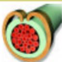
Conductors are in insulation crimp area of the contact
