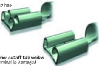
No carrier cutoff tab visible and terminal is damaged
