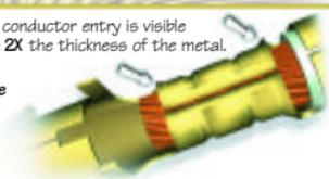
Bellmouth **only at the conductor entry end** and not at the conductor brush end of the crimp.
