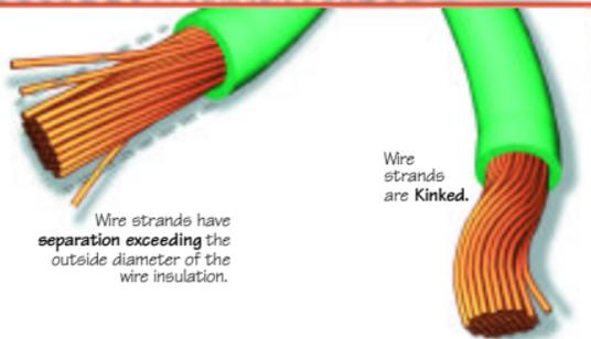
Wire strands have **separation exceeding** the outside diameter of the wire insulation.
