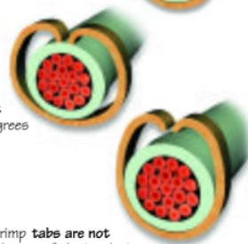
Both insulation crimp tabs are not in contact with the top of the insulation.
