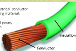
Conductors are either stranded or solid, and are usually copper or plated copper. Most of the wire used in wire harness assembly is stranded.
