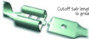
Cutoff tab length at mating end is greater than twice its thickness but does not impede mating.
