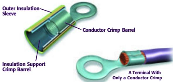
Note: All crimping needs to comply with the manufacturer's published requirements. The two methods of verifying the reliability of a crimp are by measuring the conductor crimp height and by performing a destructive pull test. Pull testing measures the force it takes to pull apart the termination between the contact and the wire.
