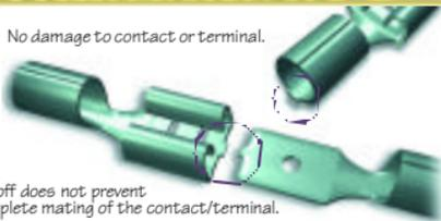
Cutoff does not prevent complete mating of the contact/terminal.
