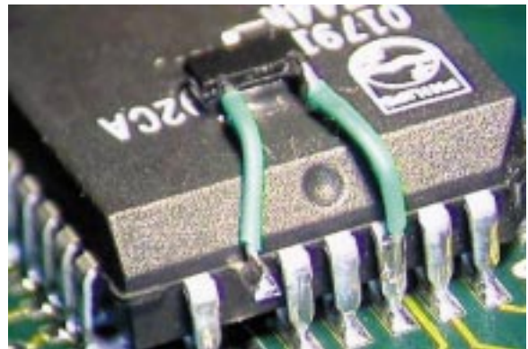
Figure 4 Chip component soldered to surface mount component using jumper wires. Note: One lead of surface mount component is shown lifted.
