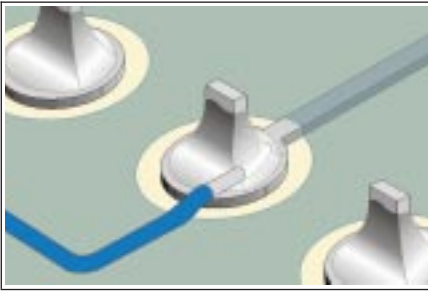
Figure 10 Acceptable Wire wrapped around component lead on solder side.
