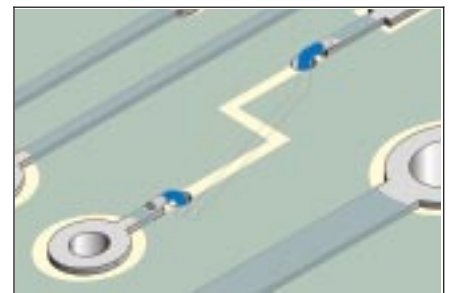
Figure 3 Drill through board, through conductors.
