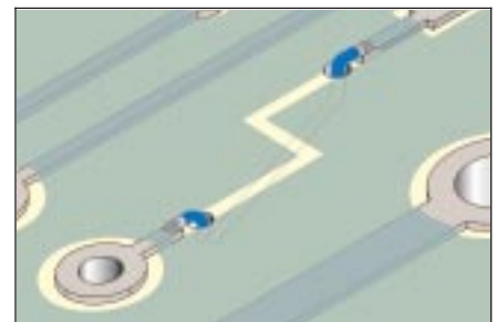
Figure 4 Lap solder wire to conductor.
