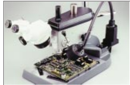
Figure 6 Sample of drill system used to cut the connection from the BGA pad to the via.
