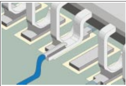
Figure 34 Not Recommended Wire soldered to lifted component lead.
