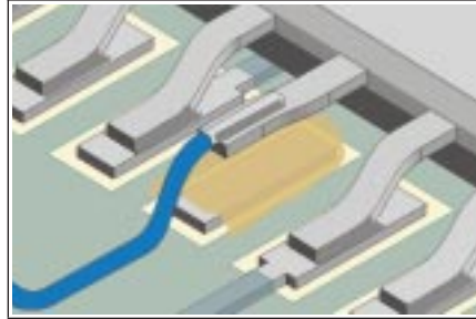
Figure 36 Acceptable Wire soldered to lifted component lead. +
