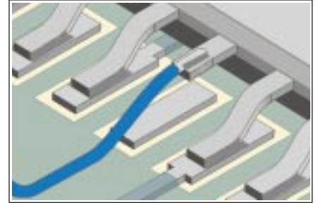
Figure 37 Acceptable Wire soldered to clipped component lead. +
